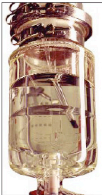
The BASIL reactor. Upper phase, the solvent-free pure product, lower phase, ionic liquid.
